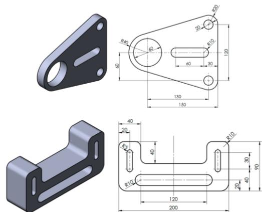
**Figure 2.** Example of the profile of model forms
