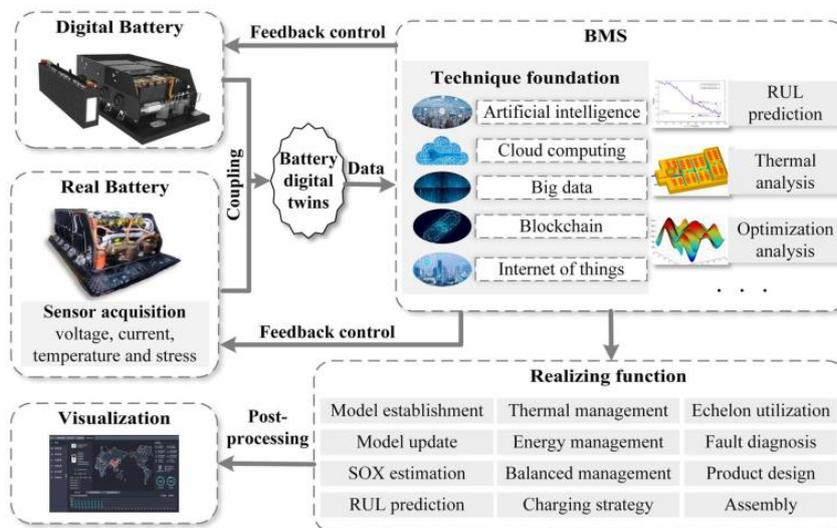
Fig. 5. Machine learning framework for DT technology in the domain of intelligent battery management systems
