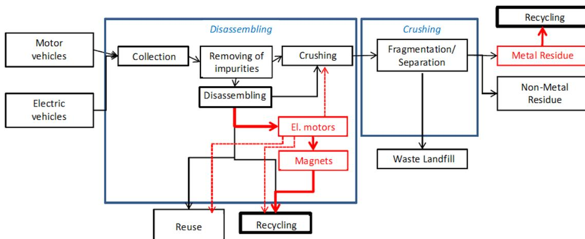
Fig. 7. Application of ML within a facility for recycling and reuse of rare magnets inside EV
