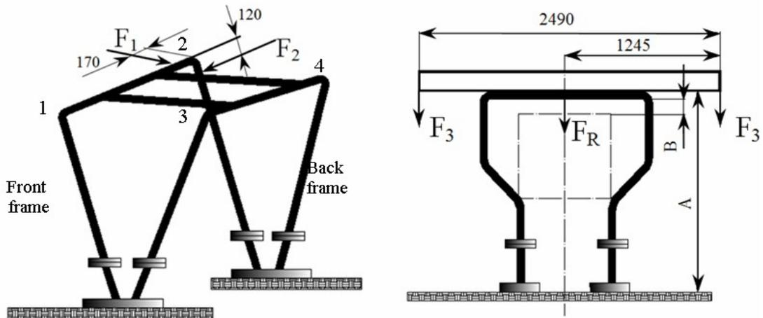
Fig. 2. Loads of protective frame
