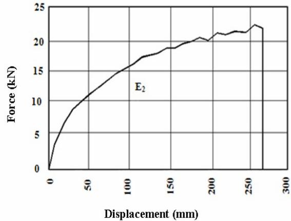
Fig. 3. Total absorbed energy of protective frame
