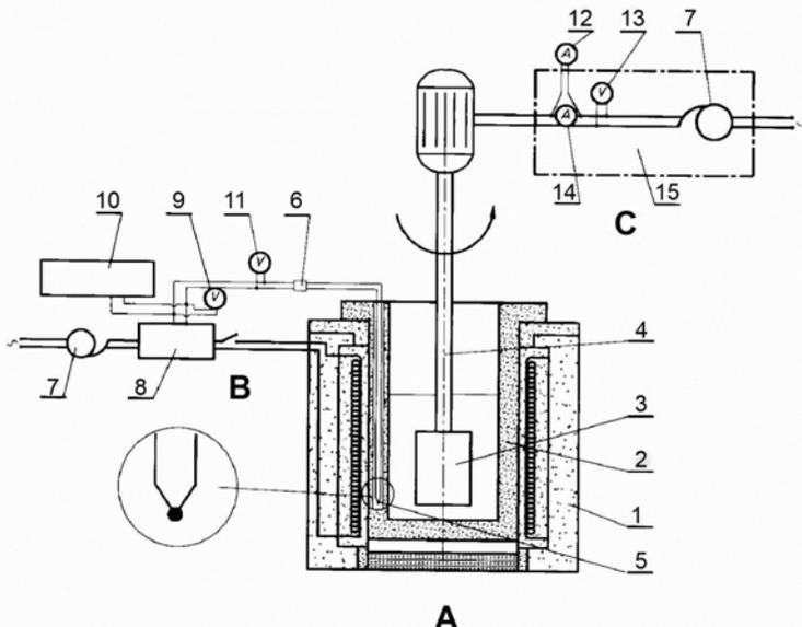
**Figure 1:** Schematical view of apparatus for rheological investigations. A. Process section; B. Control and regulation temperature section; C. section for measuring and control of electric parameters, 1. Electro resistance furnace, 2. Alumina crucible, 3. Stirrer, 4. Shaft, 5. Thermocouple.
