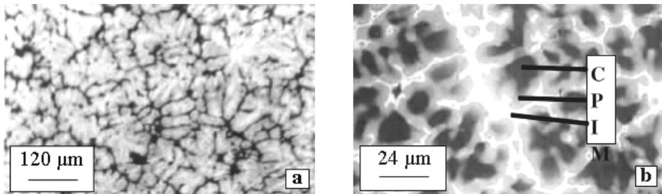
**Figure 6:** ZA27, as cast, a) OM, b) SEM, C-dendrite core, P-dendrite periphery, I-interdendritic phase.
