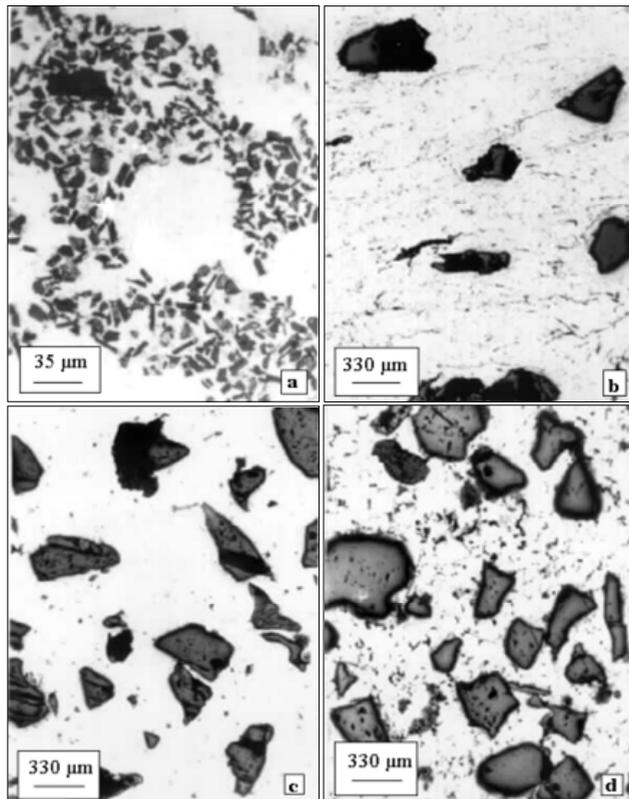
**Figure 9:** Composites (OM): a) ZA27 + 3 wt.% Al<sub>2</sub>O<sub>3</sub>, 12 μm, b) ZA27 + 3 wt.% Al<sub>2</sub>O<sub>3</sub>, 250 μm, c) ZA27+8 wt.% Al<sub>2</sub>O<sub>3</sub>, 250 μm, d) ZA27+16 wt.% Al<sub>2</sub>O<sub>3</sub>, 250 μm.
