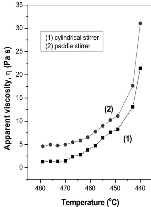
**Figure 3:** Apparent viscosity-temperature dependence of ZA27 alloy for different stirrer type. Shear rate  $132 \text{ s}^{-1}$ .
