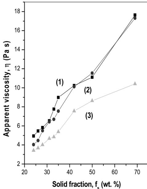
**Figure 4:** Apparent viscosity – solid fraction dependence for different reinforcing particle size. Shear rate  $132 \text{ s}^{-1}$ . Legend: 1. ZA27, 2. ZA27+3 wt.%  $Al_2O_3$ , 12  $\mu m$ , 3. ZA27+3 wt.%  $Al_2O_3$ , 250  $\mu m$ .
