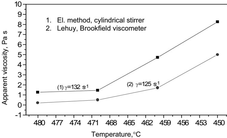
**Figure 10:** Comparison between Lehu's results and the results obtained in this work, at similar shear rate value.
