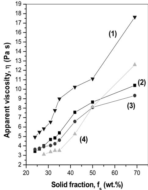
**Figure 5:** Apparent viscosity – solid fraction dependence for different mass fraction of reinforcing particles (same size). Shear rate  $132 \text{ s}^{-1}$ . Legend: 1. ZA27, 2. ZA27+3 wt.%  $Al_2O_3$ , 250  $\mu m$ , 3. ZA27+8 wt.%  $Al_2O_3$ , 250  $\mu m$ , 4. ZA27+16 wt.%  $Al_2O_3$ , 250  $\mu m$ .
