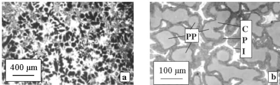
**Figure 7:** ZA27, rheo-cast, SEM. C-dendrite core, P-dendrite periphery, I-interdendritic phase, PP– primary particles.
