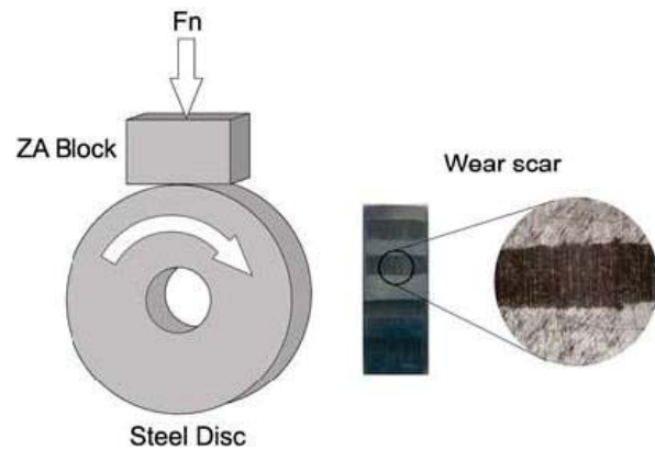
Fig. 2. The scheme of contact pair geometry
